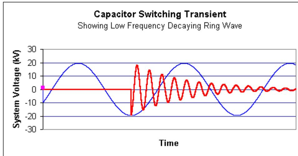
Figure 3 – Low Frequency Decaying Ring Wave Resulting From Capacitor Switching
