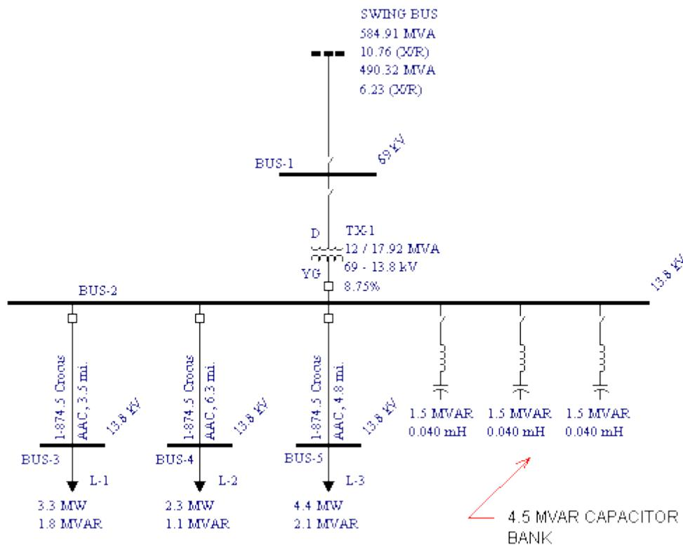
Figure 1 – Typical Utility Substation Showing a 4.5 MVAR Capacitor Bank And Adjacent Distribution Loads
