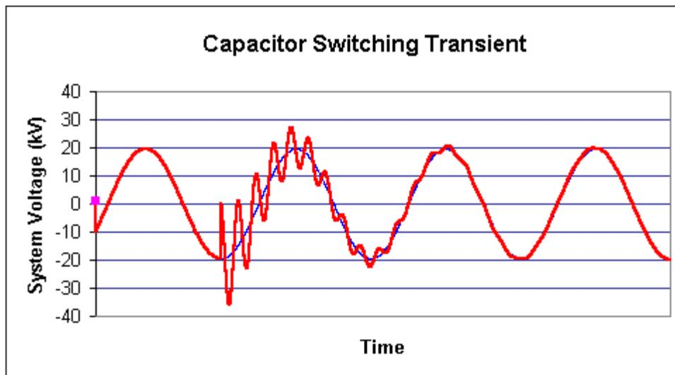
Figure 2 – Capacitor Bank Switching Transient. Bus-2 Phase-to-Phase Voltage Upon Closing of Phase-A and Phase-B Vacuum Contacts.
