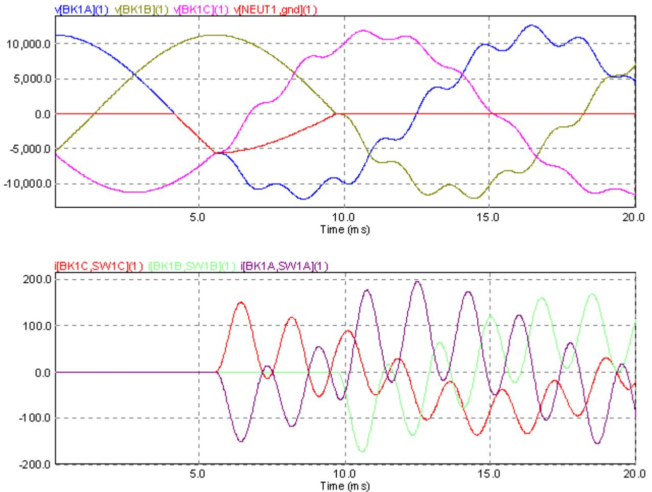
Figure 7 – Simulated Phase-to-Ground Voltage, Capacitor Bank Neutral Voltage and Vacuum Switch Current Associated with Zero-Voltage Closing
