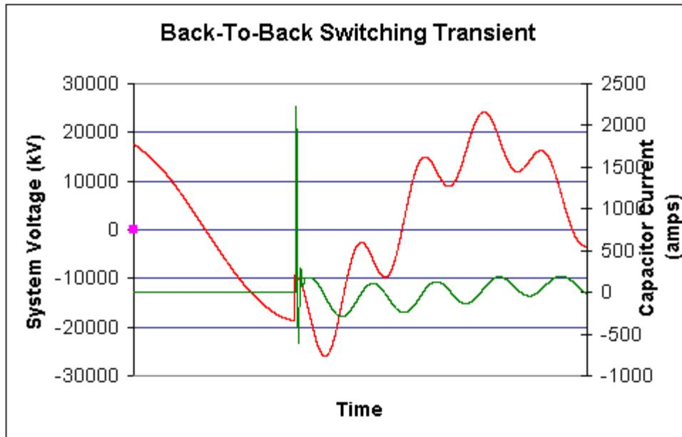
Figure 6 – Voltage (Red) and Current (Green) Waveform Associated With Back-To-Back Capacitor Bank Switching. Current Waveform Is Current Flowing Into Capacitor Bank Being Energized
